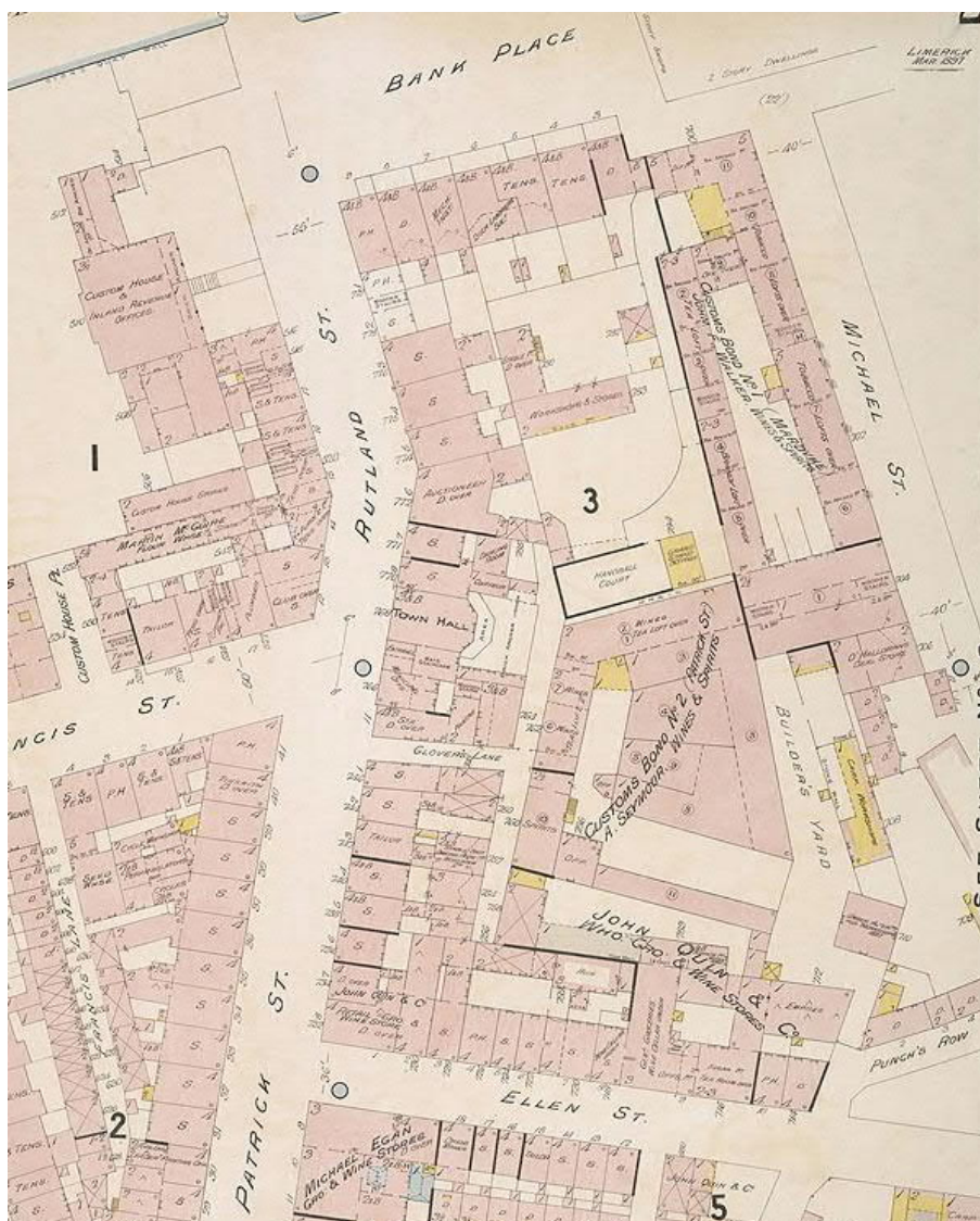
Fig. 8: Goad Insurance Plan showing the buildings to the site, 1897. Pink indicates a brick, stone or concrete building, while yellow indicates a wooden structure.
